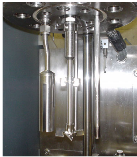
Picture 2. The inserts of the reactor (ultrasound probe, stirrer, heater, temperature sensor)
