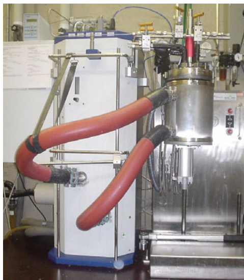
Picture 1. The reactor-calorimeter system
