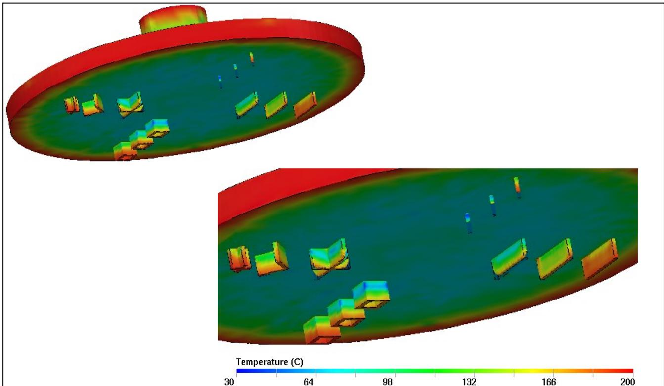
Figure 8 – Temperature distribution at the end of packing
