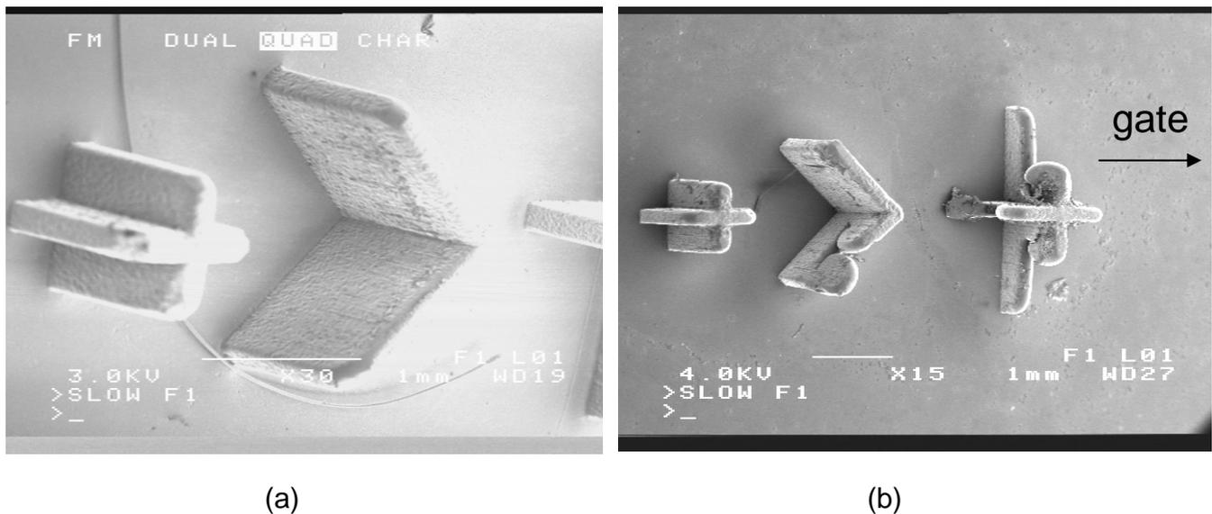
**Figure 3** – SEM micrographs of microstructures molded at the same conditions except for the mold temperature during filling: (a) 105 °C and (b) 30 °C.
