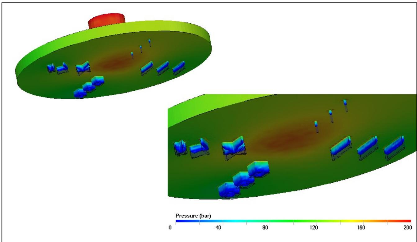
Figure 4 – Pressure distribution at the end of filling
