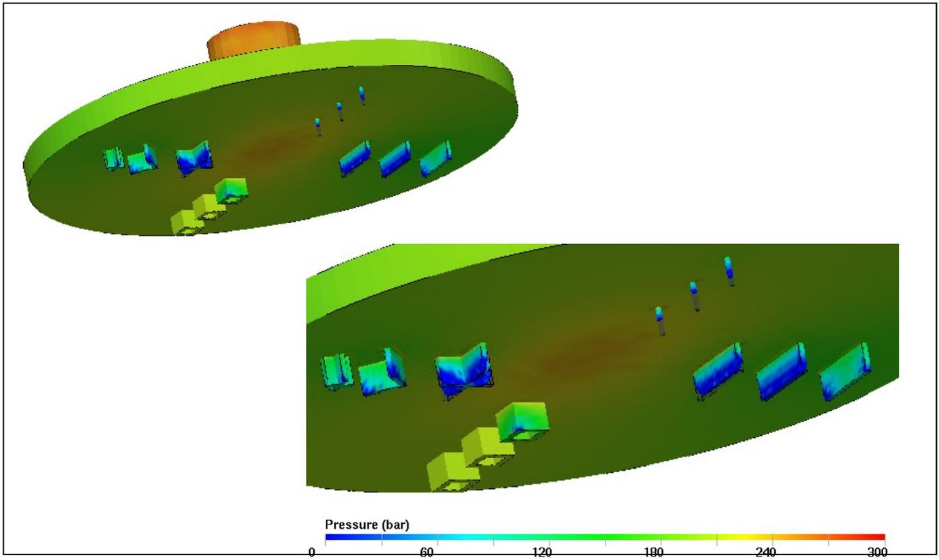
Figure 7 – Pressure distribution at the end of packing
