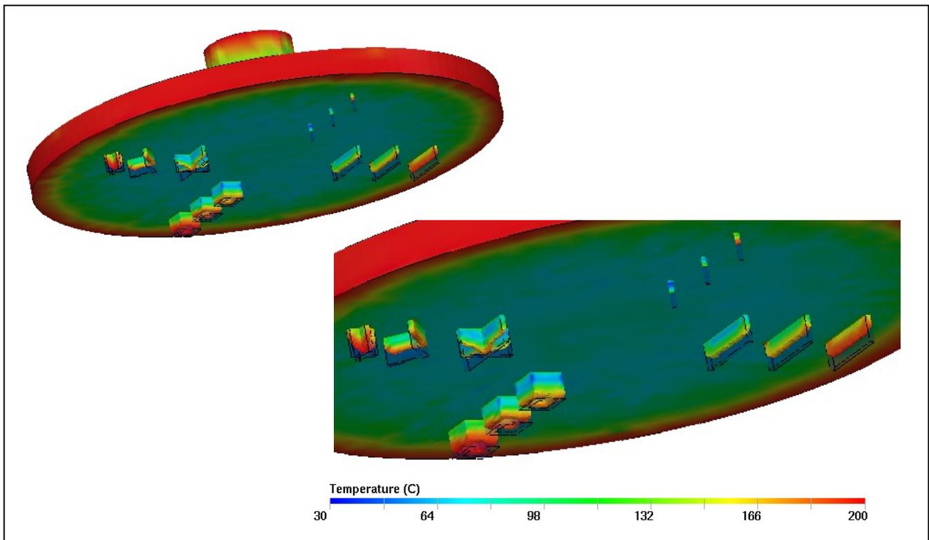
Figure 5 – Temperature distribution at the end of filling
