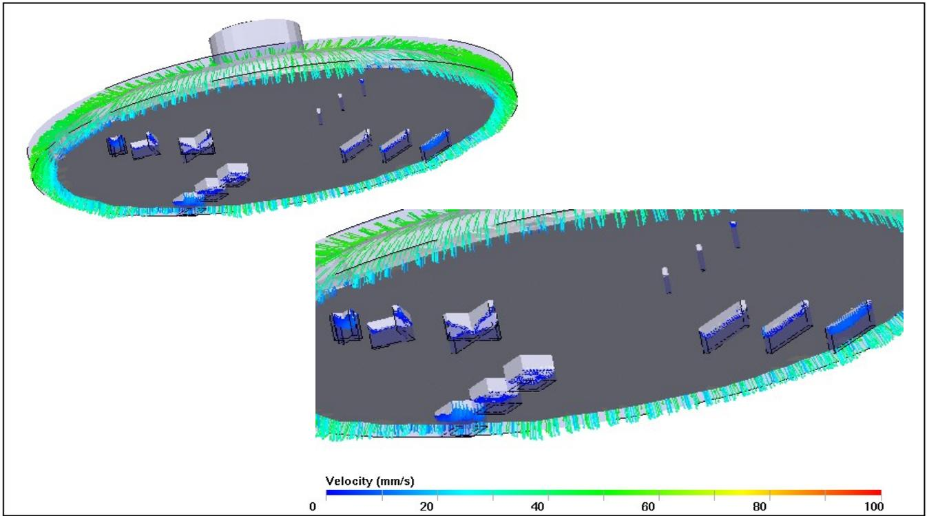
Figure 6 – Velocity distribution at the end of filling
