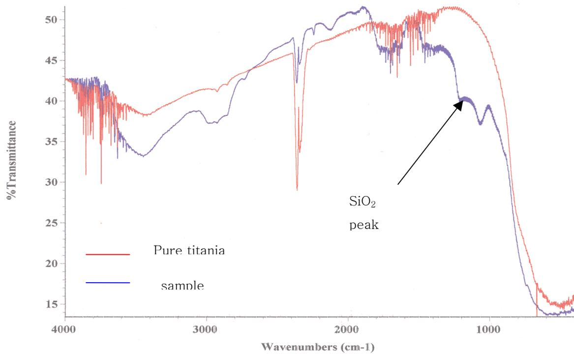
**Figure 2.** FTIR spectra of pure titania and modified titania particles
