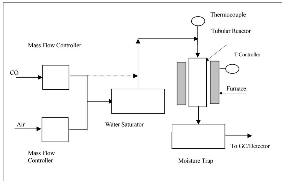
Figure 1: Schematic Diagram of CO Oxidation set-up
