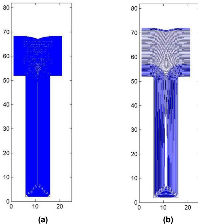
**Figure 1.** Simulations of additive-free copper electrodeposition into a  $0.15 \mu\text{m}$  trench with 5:1 aspect ratio at an applied overpotential of (a)  $-0.12 \text{ V}$  and (b)  $-0.25 \text{ V}$ . The simulation in (a) required 100 s to fill the trench and the simulation in (b) required 15.4 s to fill the trench.
