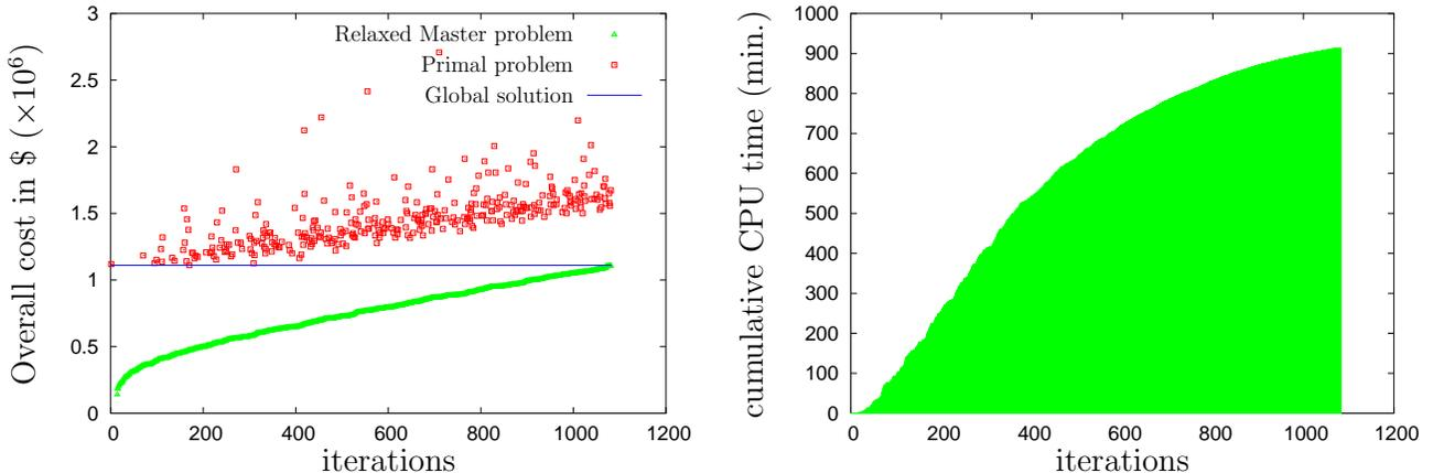
Figure 2: Case study problem — *left plot*: MIDO iterations; *right plot*: CPU time (with domain reduction).
