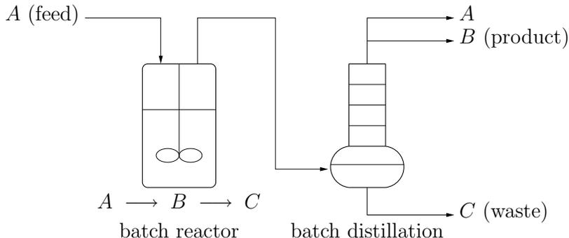
Figure 1: Task network of a 2-stage batch process.
