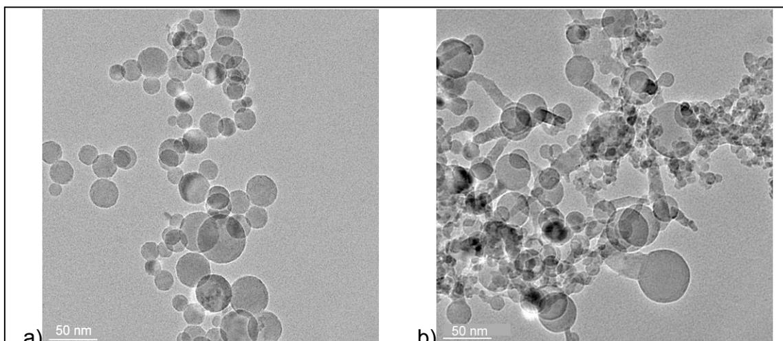
**Figure 1. Different particle morphologies produced in the plasma torch. a) spherical, and b) tailed particles**
