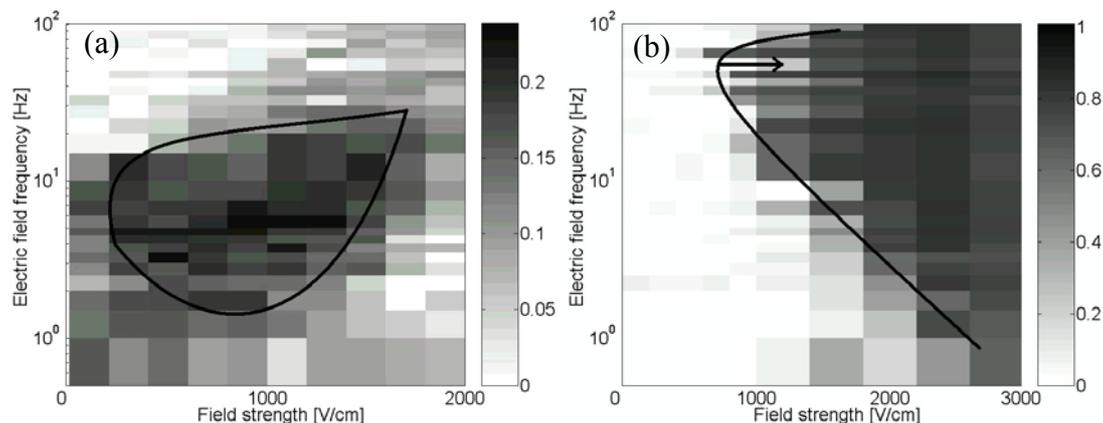
Figure 3. Bubble size decrease at 190 mm (63% of bed height). The grayscale shows the fractional change in bubble diameter as a function of frequency and field strength. Bed material: (a) 77  $\mu\text{m}$  glass beads, (b) 770  $\mu\text{m}$  glass beads. Black lines denote the region of optimal electric field strength and frequency.
