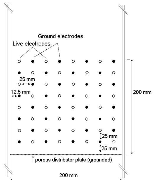
Figure 2. Schematic of the 2-D column design.
