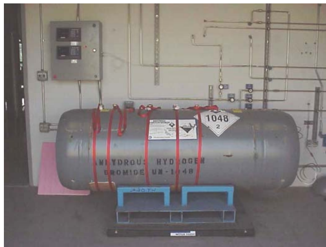
Figure 6. Experimental setup for the bulk delivery system.
