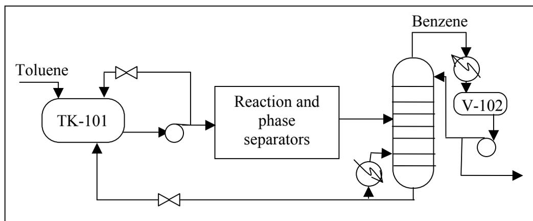
Figure 5: Diagram of the hydrodealkylation unit
