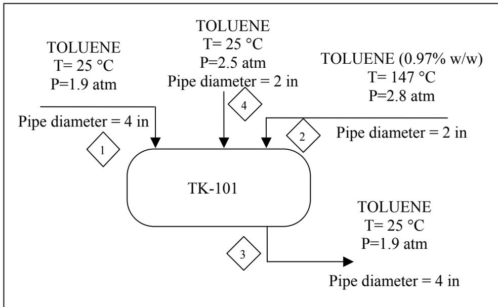
Figure 6: Diagram of the storage tank TK-101
