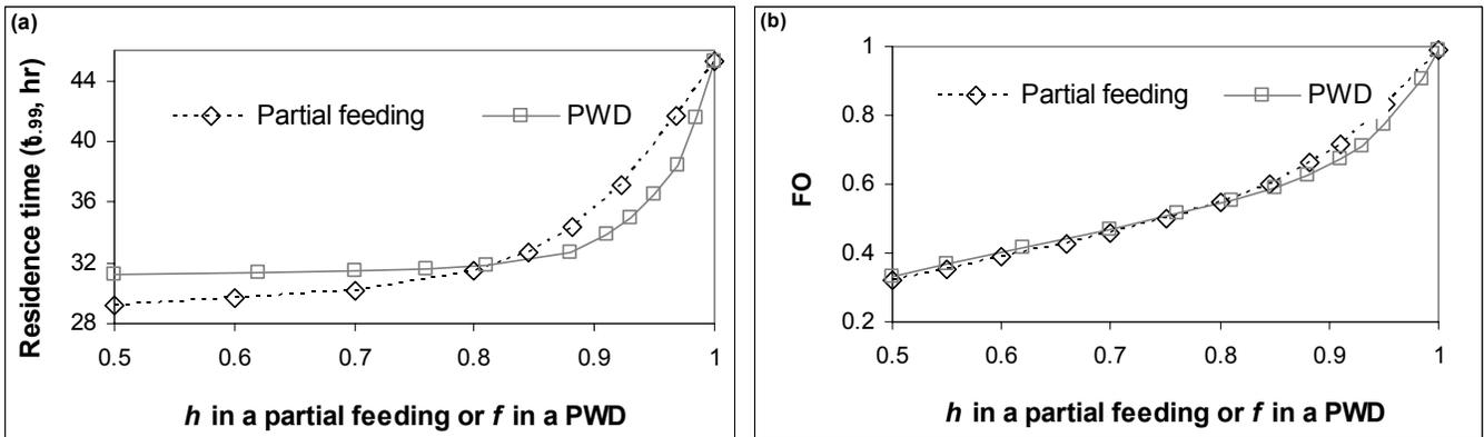
Figure 6. Partial feeding strategy and PWD method for reducing  $FO$  in Ring II. No gap is put between batch injections. (a) Effect of  $h$  or  $f$  on the residence time ( $t_{0.99}$ ) of insulin; (b) Effect of  $h$  or  $f$  on  $FO$ .
