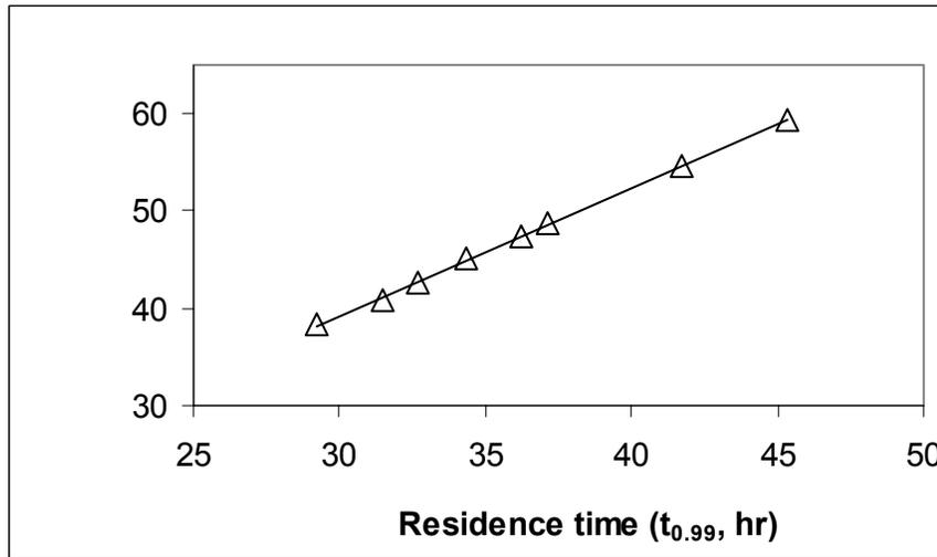
Figure 4. Correlation between  $t_{0.99}$  and  $\Delta_{feed}^{\min}$  in the second ring of a tandem SMB for insulin purification.  $t_{0.99}$  is the time that 99% of insulin have left the SMB when the feed is injected during one switching period. The y-axis is normalized by the switching time ( $t_s = 36.2$  min).
