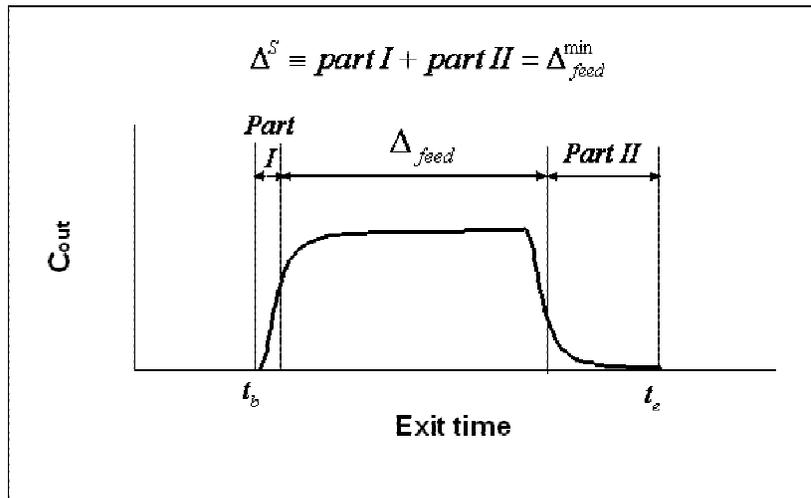
Figure 3. Representation of  $\Delta_{feed}^{min}$  in the effluent history. Concentrations in the effluent history are averaged over one switching period.
