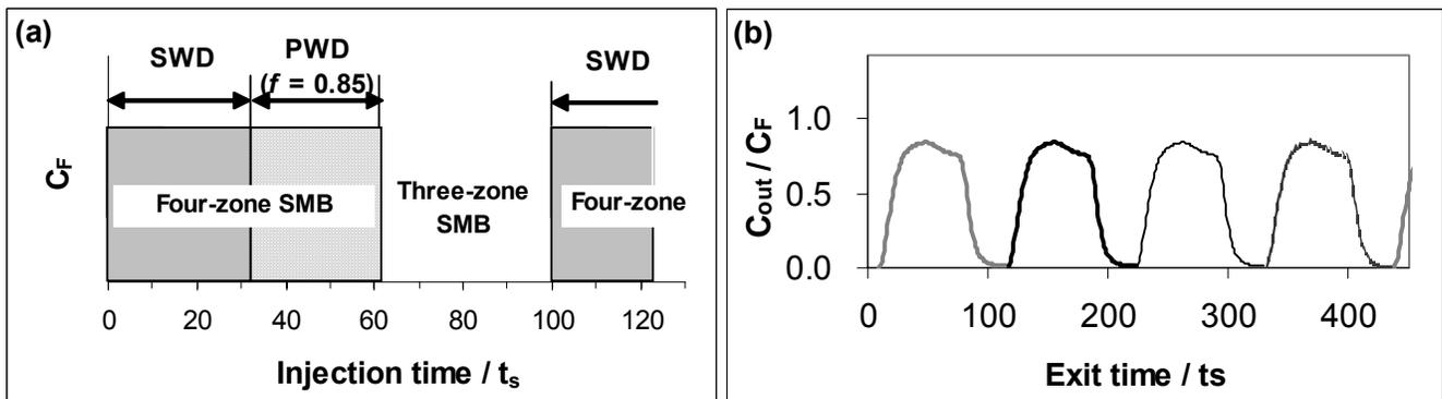
Figure 10. Alternate use of PWD ( $f = 0.85$ ), SWD, a four-zone SMB, and a three-zone SMB for complete batch integrity in Ring II. (a) Change in operation mode; (b) Effluent history of insulin at the raffinate port.
