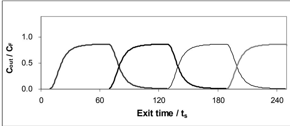
Figure 5. Effluent history of insulin from the injections of a series of batches with a size of  $60t_s$  in Ring II. Concentrations in the effluent history are averaged over one switching period.
