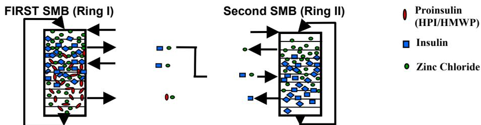
Figure 1. Schematic of a tandem SMB process for insulin purification.
