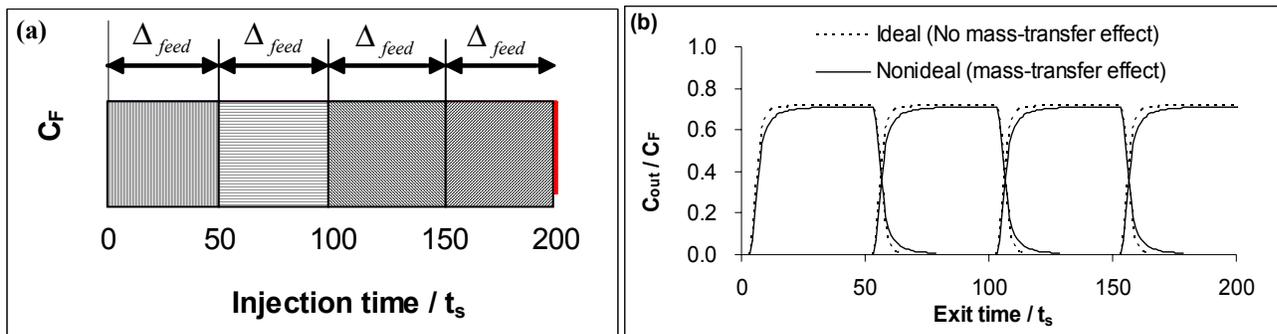
Figure 2. Batch integrity in the first ring of a tandem SMB for insulin purification. (a) Injections of a series of feed batches with a size of 50 t<sub>s</sub>; (b) Effluent history of insulin at the extract port. Concentrations in the effluent history are averaged over one switching period.
