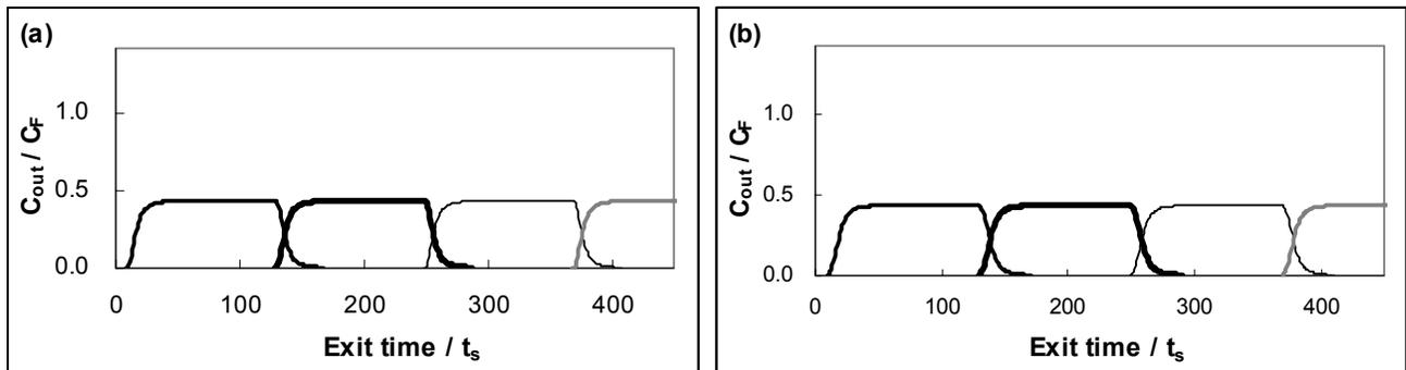
Figure 7. Effluent histories of insulin from the strategies to reduce  $FO$  in Ring II. (a) Partial feeding ( $h = 0.5$ ) without a gap; (b) PWD ( $f = 0.5$ ) without a gap
