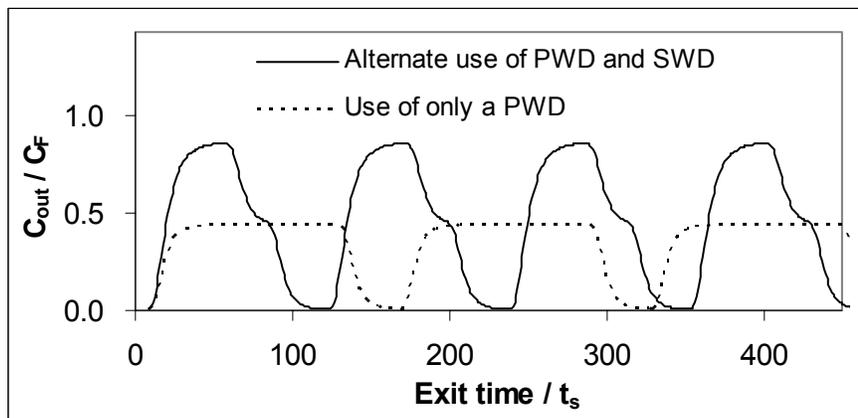
Figure 9. Comparison of the effluent histories of insulin in Ring II from the alternate use of PWD ( $f = 0.5$ ) & SWD and the use of only PWD ( $f = 0.5$ ). An eluent gap with a size of  $40t_s$  is injected between two adjacent batches.
