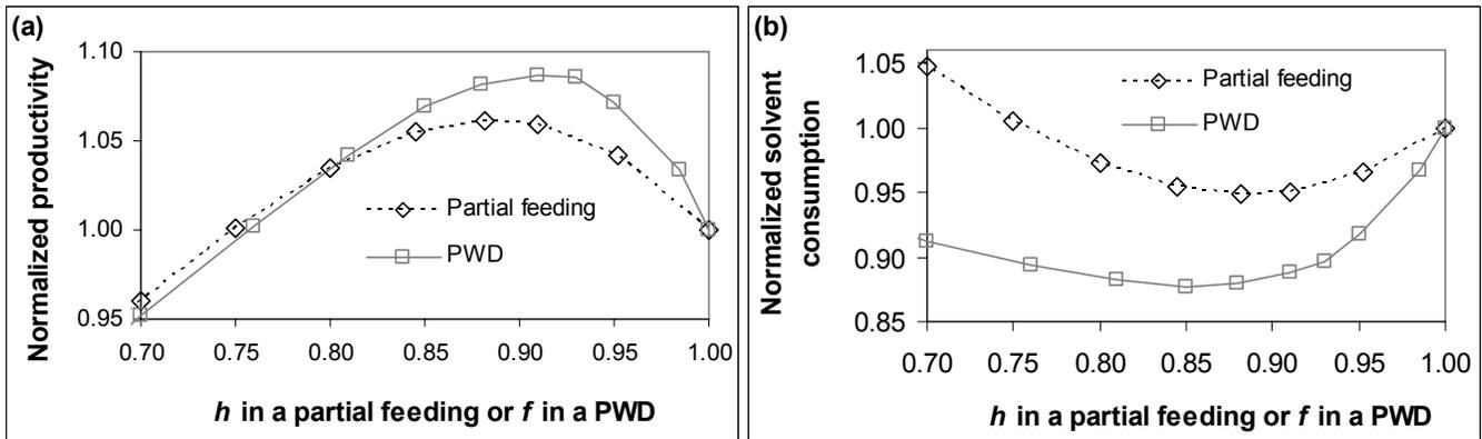
Figure 8. Partial feeding strategy and PWD method for complete batch integrity ( $FO = 0$ ) in Ring II. A minimal eluent gap is used between batch injections. (a) Effect of  $h$  or  $f$  on productivity; (b) Effect of  $h$  or  $f$  on solvent consumption.
