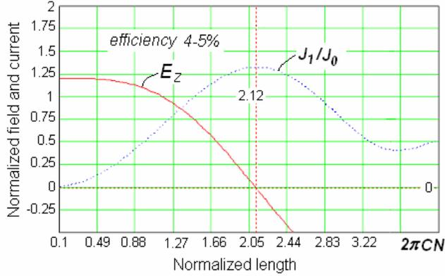
**Figure 5.** Distribution of the relative field intensity  $E_z$  and the ratio the first harmonic of the beam current  $I_1$  to the average beam current  $I_0$ .
