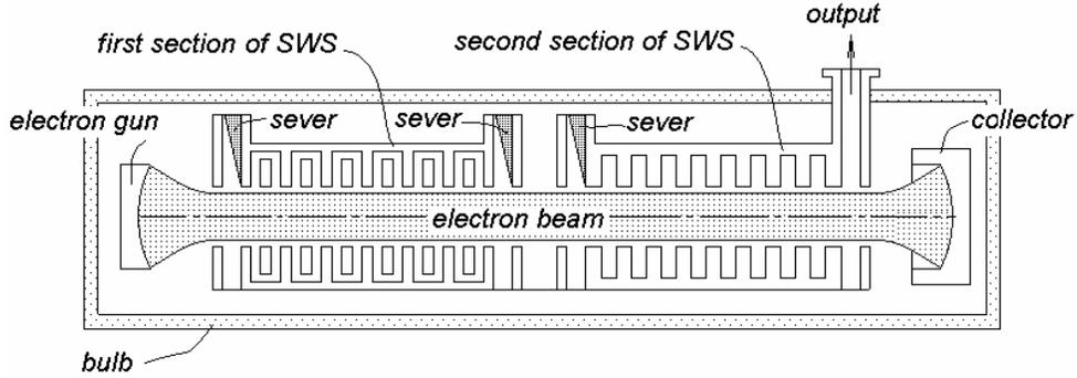
**Figure 4.** Backward-wave oscillator with BWO and TWT sections.
