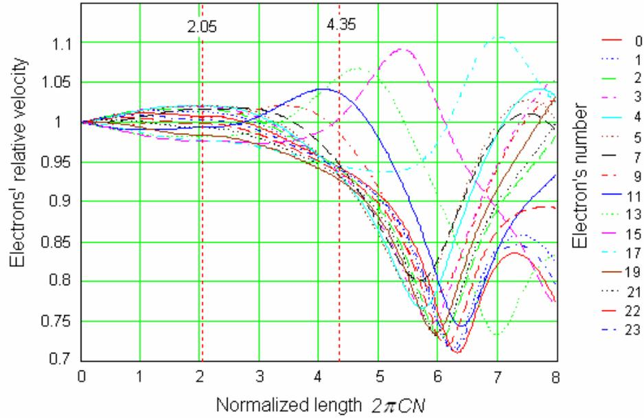
Figure 7. Phase trajectories for electrons in two-section BWO.
