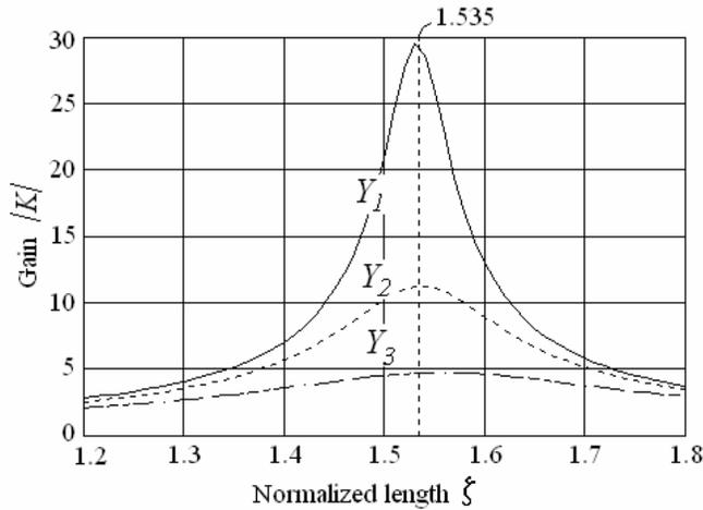
**Figure 2.** Gain factor  $K$  dependence on the normalized length calculated for three different values of the feedback coefficient.
