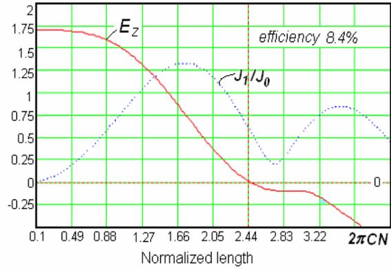
**Figure 6.** Distribution of the relative field intensity  $E_z$  and the ratio of the first harmonic of the beam current  $I_1$  to the average beam current  $I_0$  at the first section in the case of the maximum efficiency.
