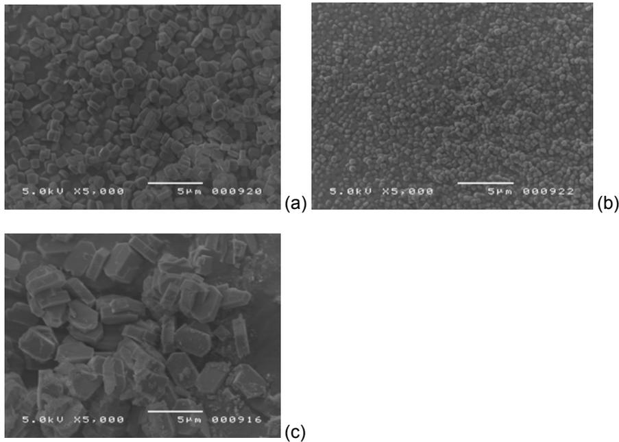
**Figure 1.** Scanning electron micrographs of silicalite from microwave synthesis with (a) 2 min ramp, 10 hold at 175°C, (b) 120 min ramp, 10 hold at 175°C and (c). 2 min ramp, 128 hold at 175°C
