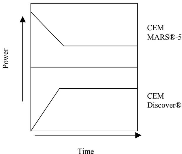
**Figure 2.** Schematic of the power versus time plot observed for MARS®-5 multi-node microwave oven and Discover® single-node microwave oven
