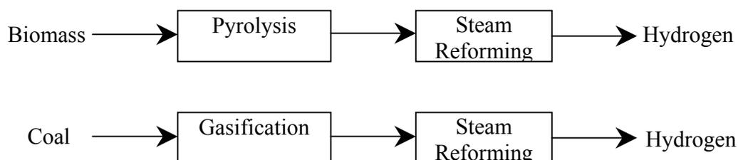
Figure 1 Conversion Process from Biomass and Coal to Hydrogen
