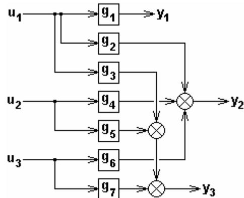
Fig. 8. Simplified Block Diagram of the Controlled Industrial Milling Circuit.
