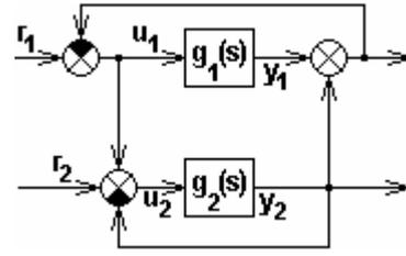
Fig. 7. The third system structure. A multivariable MIMO interconnection.
