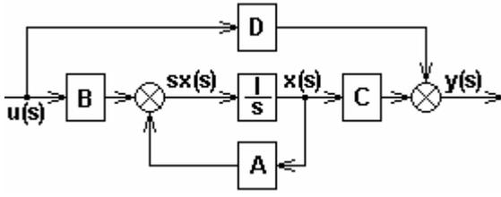
Fig. 1. Block diagram of the state space model.
