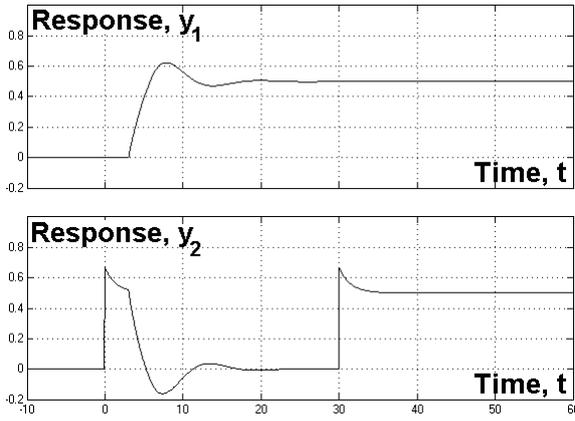
Fig. 6. Closed loop step response for the second system structure.
