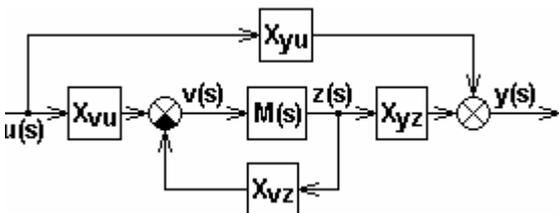
Fig. 2. Block diagram of the proposed TFCM model.
