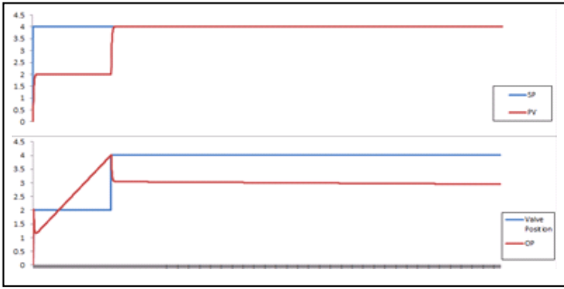
Figure 7. Detuned integral action – resulting in stable behavior.
