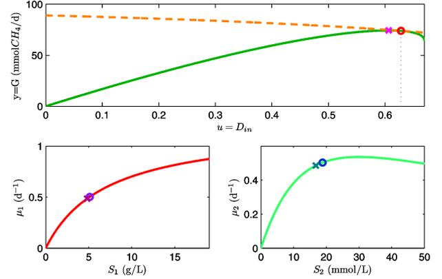
Fig. 1. Top: input/output steady state (green solid) and maximum value of  $r_y$  for fixed steady state  $S_1$  (orange dashed), showing optimal (cross) and STC feedback (circle) steady states. Bottom: specific COD and VFA consumption rates, i.e. Monod and Haldane curves.
