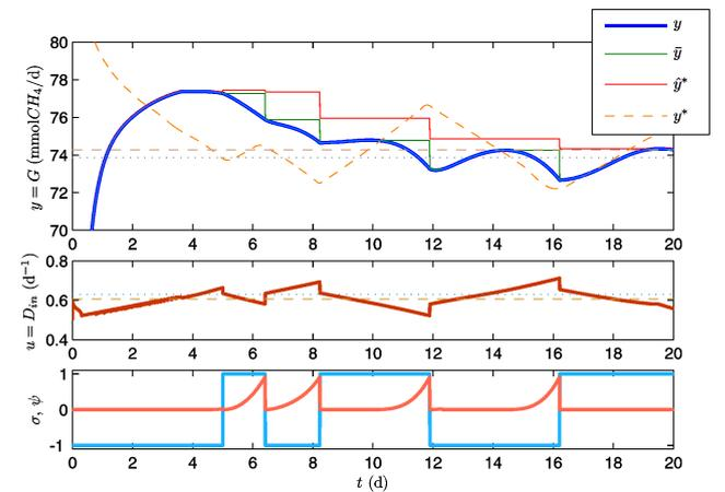
Fig. 3. Trajectories of the output and input signals without noise. Top: evolution of signals true  $y(t)$  (dark blue), noisy  $y(t)$  (light blue)  $\bar{y}(t)$  (green),  $\hat{y}^*(t)$  (red) and  $y^*(t)$  (orange). Middle: input  $u(t)$ . Bottom:  $\psi(t)$  (blue) and sign estimate  $\sigma(t)$  (orange).
