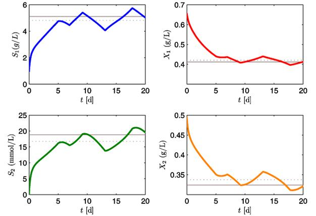
Fig. 2. Trajectories of the states in closed loop without noise.
