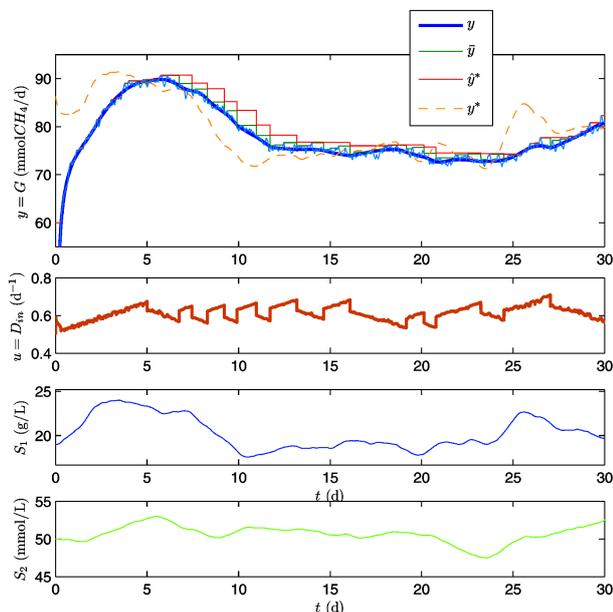
Fig. 4. Trajectories of the output and input signals with noise. Top: evolution of signals  $y(t)$  (blue),  $\bar{y}(t)$  (green),  $\hat{y}^*(t)$  (red) and  $y^*(t)$  (orange). Middle: input  $u(t)$ . Bottom graphs:  $S_1^{\text{in}}(t)$  (blue) and  $S_2^{\text{in}}(t)$  (green), respectively.
