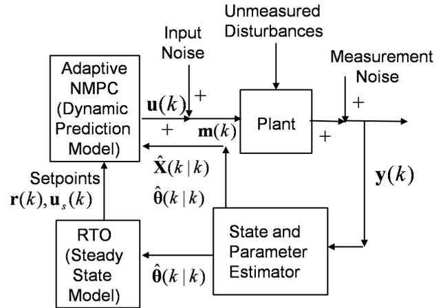
Fig. 1. Schematic Representation of the proposed integrated RTO and Adaptive NMPC Formulation
