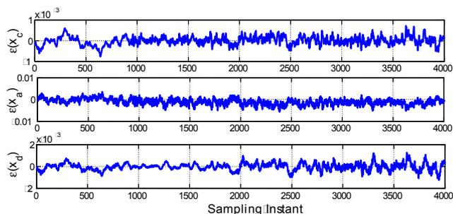
Fig. 3. Case A: Profile of state estimation errors in controlled variables
