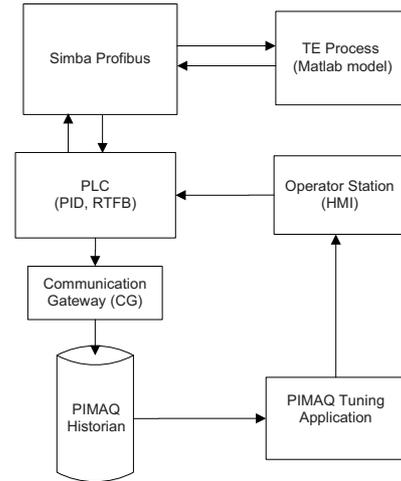
Fig. 1. Information flow in the test setup
