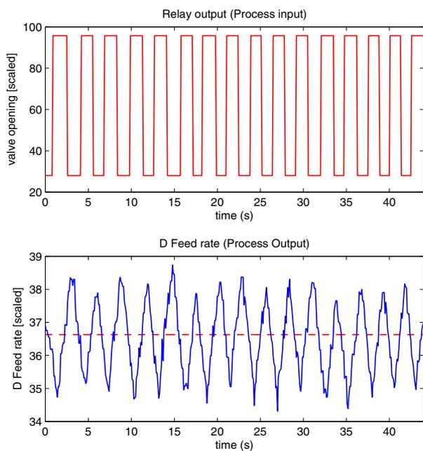
Fig. 3. Tuning data for D feed rate
