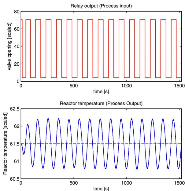
Fig. 4. Tuning data for Reactor temperature
