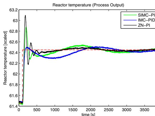
Fig. 5. Response of reactor temperature to a step in setpoint with different controllers given in Table 4
