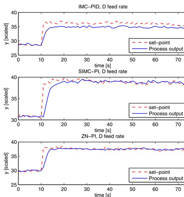
Fig. 6. Response of D feed rate to a step in setpoint with different controllers given in Table 4
