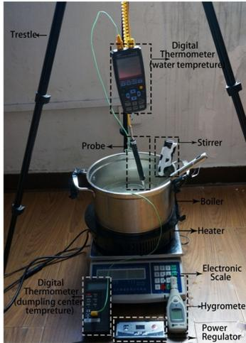
Fig. 4. Experiment setup
