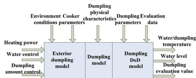
Fig. 1. System model with input, output, and working parameters
