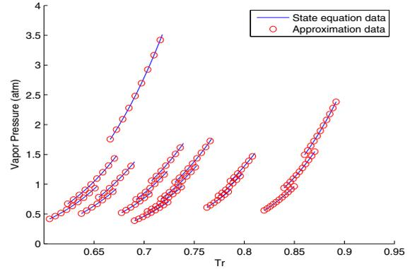
Fig. 3. The comparison of state equation data and its quadratic function approximation for different pseudo-components.
