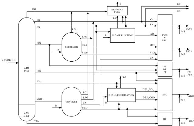
Fig. 1. A simplified refinery model flow chart in Favennec (2001).
