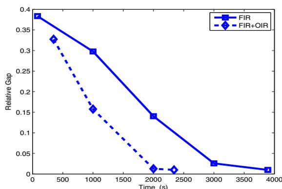
Fig. 4. The comparison of relative gap based on different interval reduction techniques
