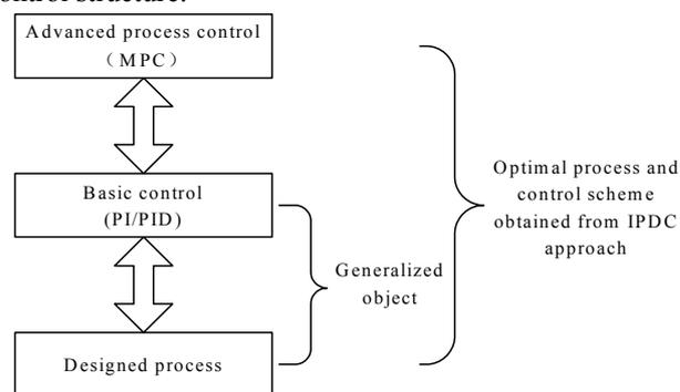
Fig. 1 IPDC framework using hierarchical control structure
