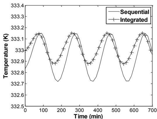
Fig. 3. Comparison of the reactive temperature using sequential and integrated design/control strategies.
