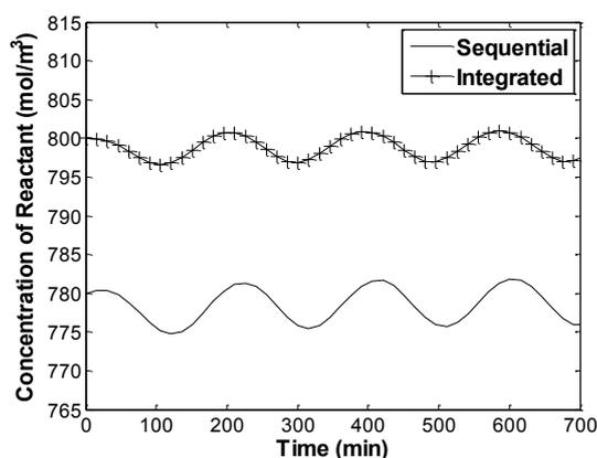
Fig. 4. Comparison of the concentration of reactant using sequential and integrated design/control strategies.
