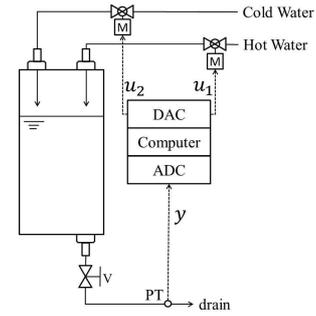
Fig. 9. Schematic figure of temperature control system.
