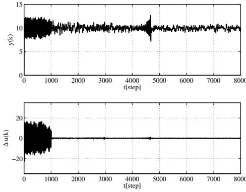
Fig. 3. Control result by proposed control scheme in the case of  $\sigma_e^2 = 0.4$ .
