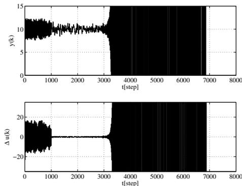
Fig. 8. Control result using the fixed PID parameters which are tuned by the ZN method.
