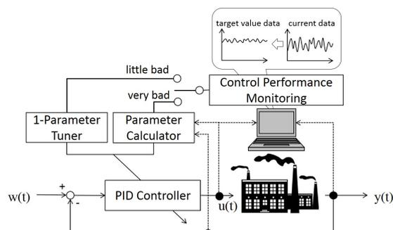
Fig. 1. Schematic diagram of the smart adaptive controller.
