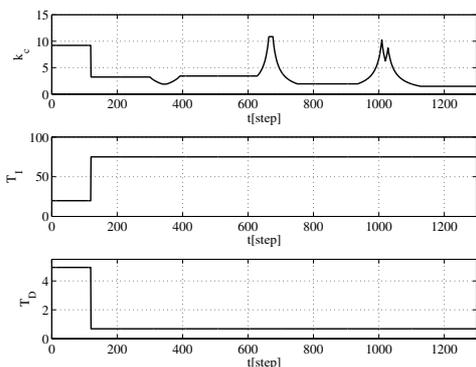
Fig. 11. Trajectories of PID parameters corresponding to Fig. 10.
