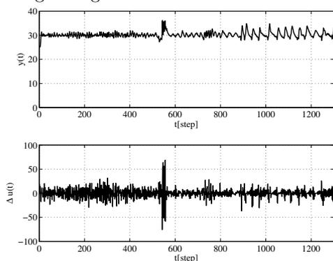
Fig. 14. Control result using the fixed PID parameters which are tuned by the ZN method.
