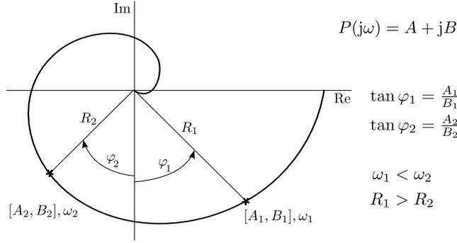
Fig. 5. System transfer function computation from two points of frequency response
