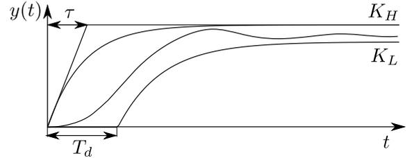
Fig. 4. *A priori* process knowledge for evaluation of error in computing process frequency response samples: residual time constant  $\tau$ , maximum delay  $T_d$ , static gain limits  $K_L$ ,  $K_H$
