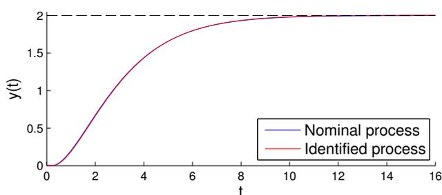
Fig. 11. Example 2 – Comparison of nominal and identified process step responses
