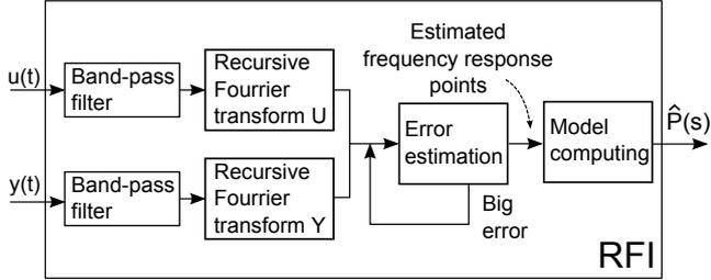
Fig. 3. General structure of RFI block with process frequency response estimator based on RDFT
