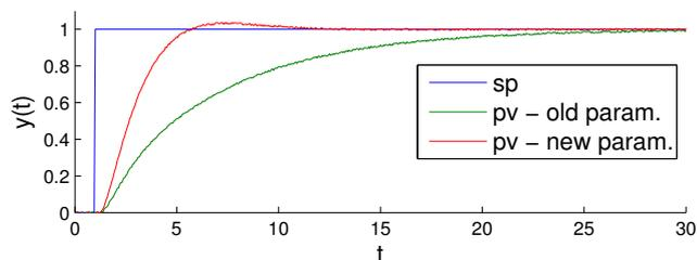
Fig. 15. Example 2 – Closed loop system step response
