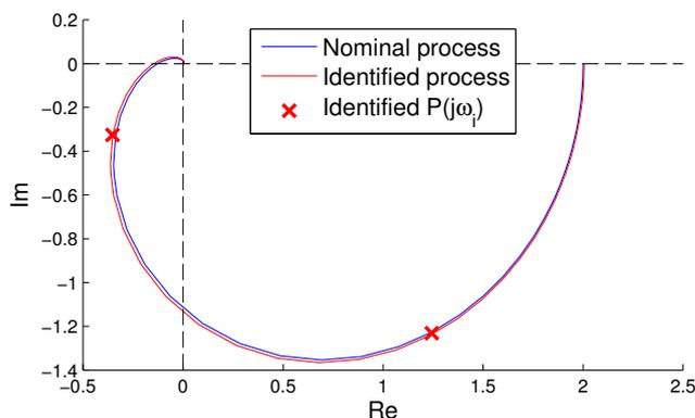
Fig. 10. Example 2 – Nyquist plots of nominal and identified process with estimated frequency response points
