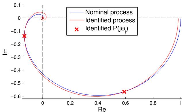
Fig. 7. Example 1 – Nyquist plots of nominal and identified process with estimated frequency response points
