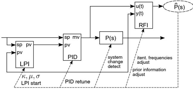
Fig. 2. Control loop performance assessment and system close-loop identification scheme
