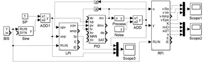
Fig. 6. Scheme of simultaneous loop performance index and frequency response points estimation algorithm
