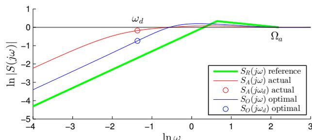
Fig. 14. Example 2 – Sensitivity functions comparison;  $\Omega_a = 9 \text{ rad} \cdot \text{s}^{-1}$ ,  $\omega_d = 2.55 \text{ rad} \cdot \text{s}^{-1}$ ,  $A_d = 0.05$ .
