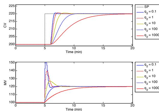
Fig. 1. Setpoint change for SISO MPC for different MV movement cost weight ( $q_2$ )
