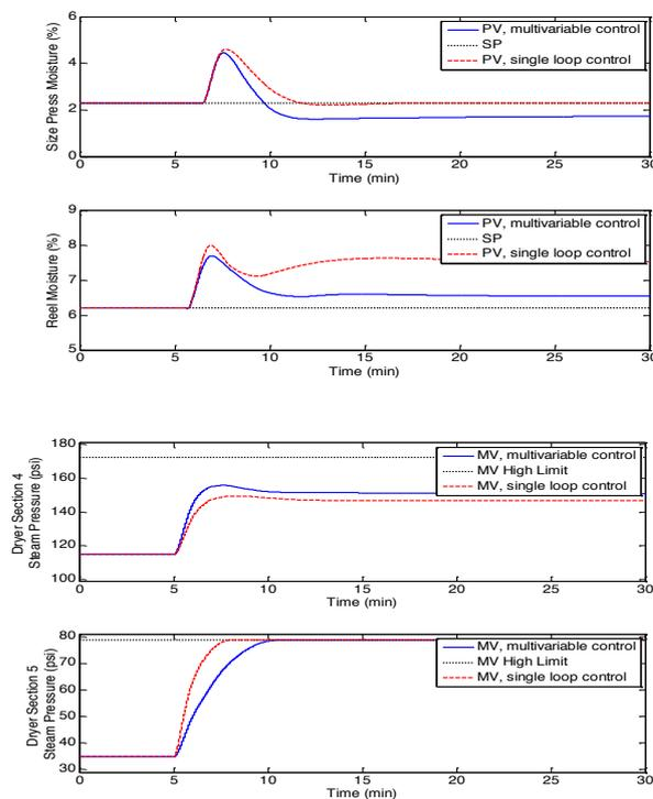
Fig. 2. CV movements for single loop and MPC control.
