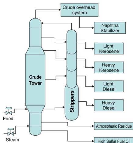
Fig. 2. A systematic sketch of an atmospheric column unit.
