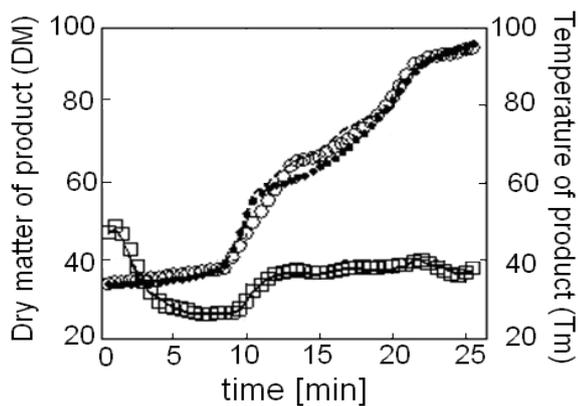
Fig. 5. The simulation results of the ANN based model. *DM* experimental, (o) *DM* simulation (---),  $\Delta DM$  simulation (●●), *T<sub>m</sub>* experimental (□), *T<sub>m</sub>* simulation (—).
