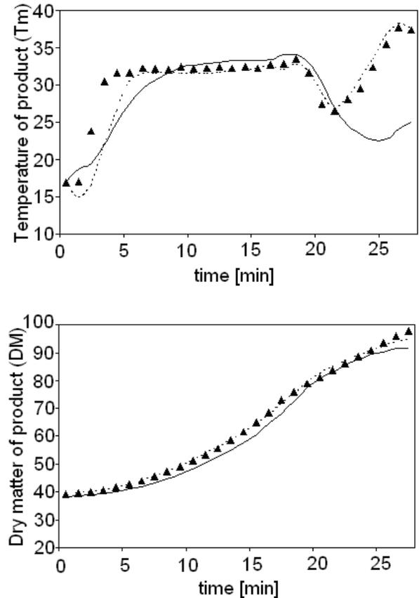
Fig. 4. Simulation results of the energy and mass balance based model (—) and granule based model (---). Industrial data ( $\blacktriangle$ ).
