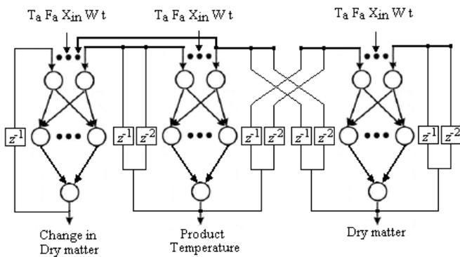
Fig.1. Drying model architecture designed using recurrent ANN.  $t$ : the drying time (s),  $W$ : loading (kg),  $X_{in}$ : moisture content of inlet air (kg water/kg air),  $F_a$ : flow rate of inlet air ( $m^3/h$ ) and  $T_a$ : temperature of inlet air (°C).
