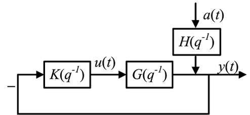
Fig. 2. Block diagram of closed-loop system
