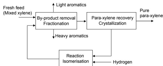
Fig. 1. Typical para-xylene production process
