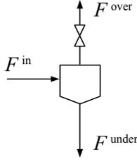
Fig. 3. Hydrocyclone separator modeling
