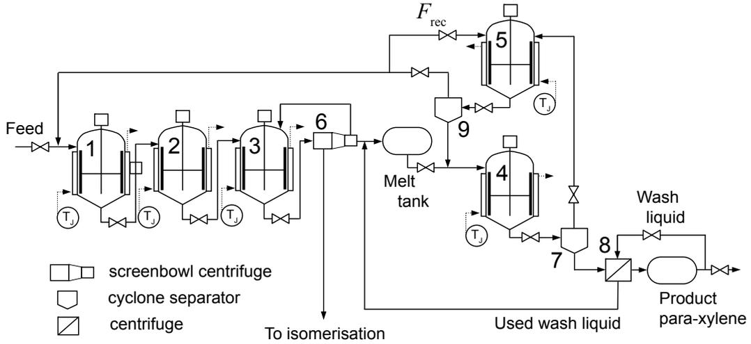
Fig. 2. Process flow of the para-xylene recovery section. The numbers (1 ~ 9) denote the equipment numbers which are used as subscript to distinguish the equipments.
