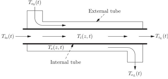
Fig. 1. co-current heat exchanger.
