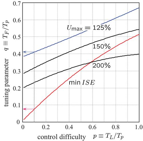
Fig. 5. Tuning of robust I-PD controllers
