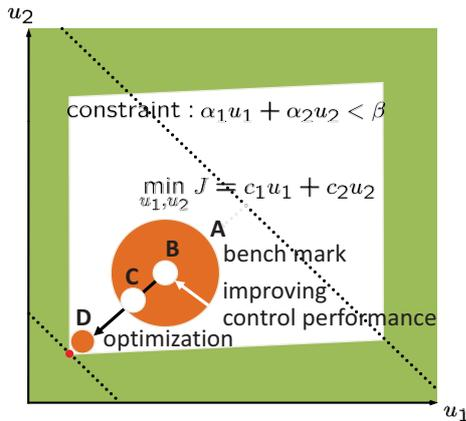
(b) optimal operation using MPC
