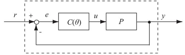
Fig. 6. Feedback control system
