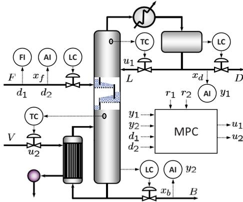
(a) MPC for distillation column
