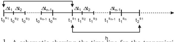
Fig. 1. A schematic showing the time-line for the transmission of each sensor suite in an  $h$ -periodic schedule.
