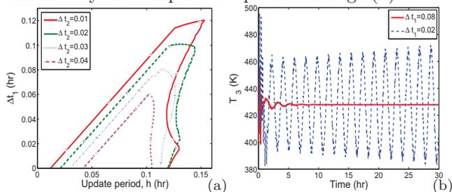
Fig. 3. (a) Dependence of  $\lambda_{\max}(M_o)$  on  $\Delta t_1$  and  $h$  for different values of  $\Delta t_2$  under schedule 2 with a fixed model, and (b) Closed-loop temperature profile for CSTR 3 when  $\Delta t_2 = 0.02$  hr and  $h = 0.13$  hr for two different values of  $\Delta t_1$ .
