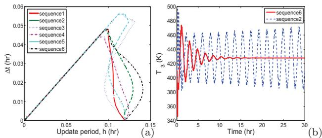
Fig. 2. (a) Dependence of  $\lambda_{\max}(M_o)$  on  $\Delta t$  and  $h$  for different sensor transmission sequences under a model-based control scheme. (b) Closed-loop temperature profile for CSTR3 under the model-based quasi-decentralized output feedback control strategy using two different sensor transmission schedules with the same update period.
