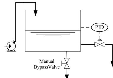
Fig. 3. Pilot scale tank process
