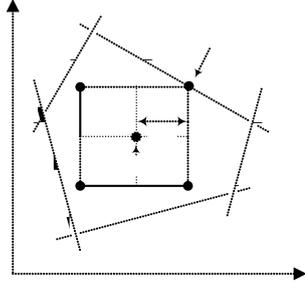
Fig. 4. Geometric representation of vertex-based flexibility target.
