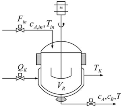
Fig. 5. Continuous Stirred Tank Reactor
