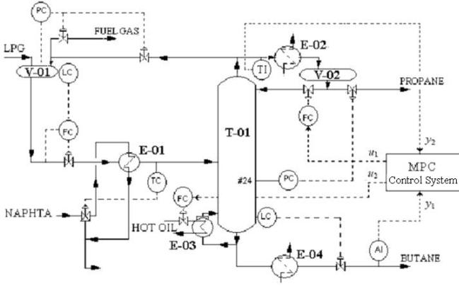
Fig. 2. Schematic diagram of the depropanizer column
