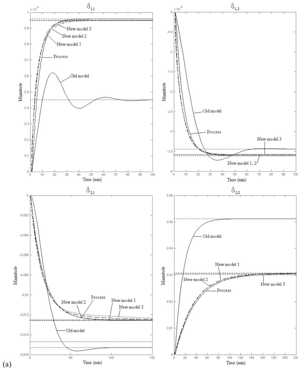
Fig. 3. Step response for the depropanizer column
