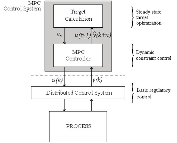
Fig. 1. Two-layer MPC structure
