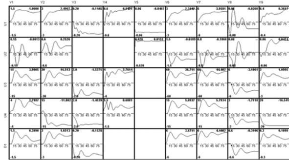
Fig. 7. Step Response Model for the SMR Problem. Responses for outputs  $y_1 - y_9$  to a step in inputs  $u_1 - u_4$  and disturbance  $d_1$ . Empty boxes represent that there is no interaction between the input-output or disturbance-output pair.
