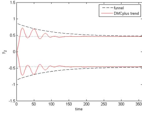
Fig. 6. Funnel Design and DMCplus trend for output  $y_2$  with  $(\alpha_f, \beta_f) = (0, -0.74)$ .
