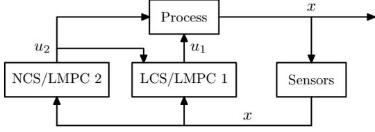
Fig. 1. Distributed LMPC design for networked control systems with continuous measurements (i.e.,  $x(t)$  is available to the controllers at  $t_k = t_{k-1} + \Delta$  where  $\Delta$  is a fixed sampling time for all  $k$ ).
