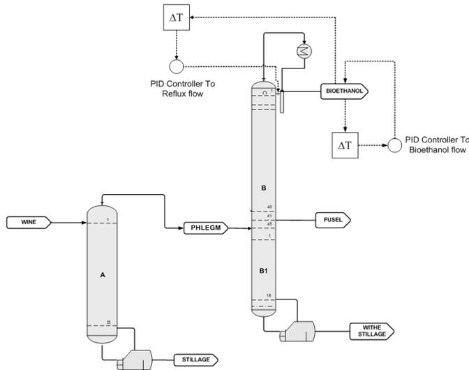
Fig. 5. Loop control for acetaldehyde concentration in bioethanol
