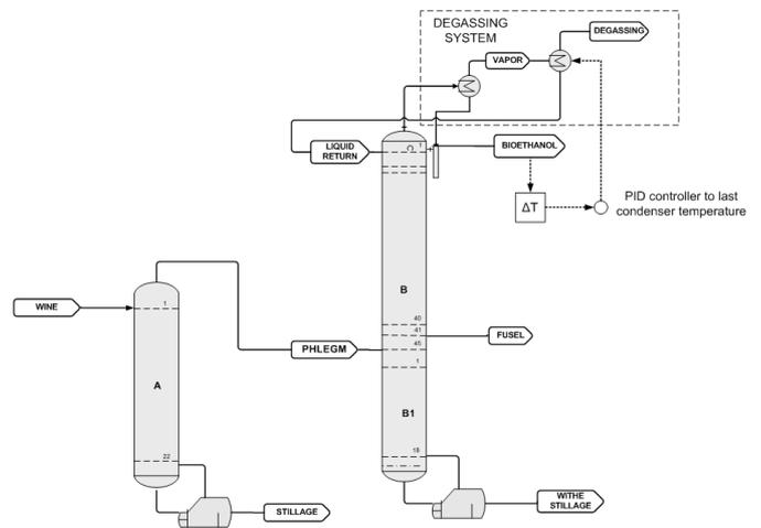
Fig. 6. Industrial plant with degassing system
