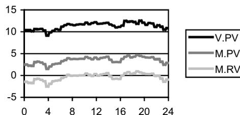
Fig. 3. Fulfilment of general mass balance (relative error [%] vs time [hr]); volumetric flow (measured process variables) and mass flow (calculated and reconciled process variables).
