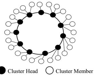
Figure 4: Federated sensor network architecture
