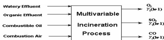
Fig. 2. Incineration system
