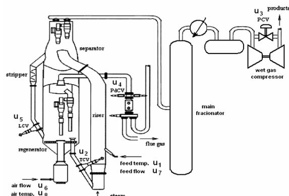
Fig. 1 FCC UOP Stacked Converter (Secchi *et al.*, 2001).
