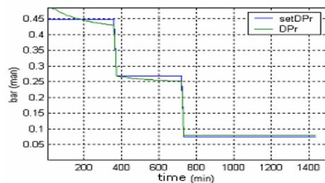
Fig. 6 Differential pressure reactor/regenerator ( $u_4$ ).
