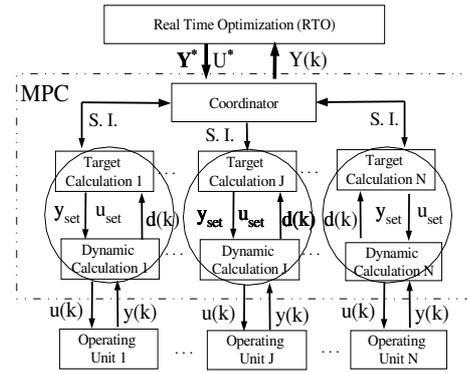
Fig. 3. coordinated, decentralized MPC target calculation
