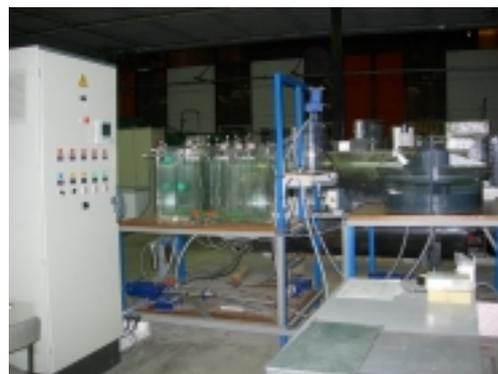
Fig. 1. The activated sludge pilot plant.
