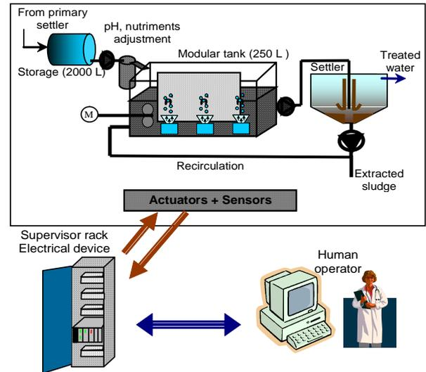
Fig. 2. Schematic representation of the pilot plant.
