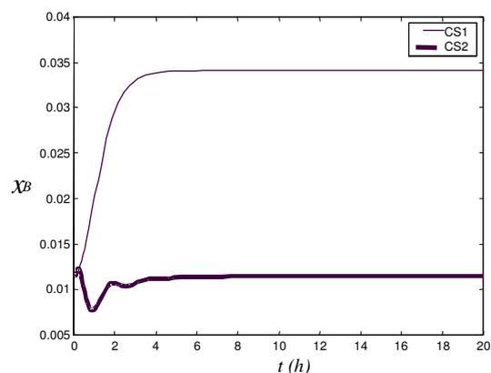
**Fig. 8.** Dynamic performances of control structures CS1 and CS2 when 10% of the feed composition is increased.
