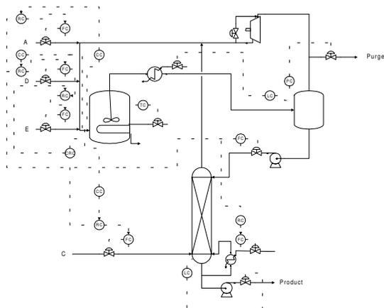
**Fig. 11.** Flowsheet of the control structure TE-CS2.
