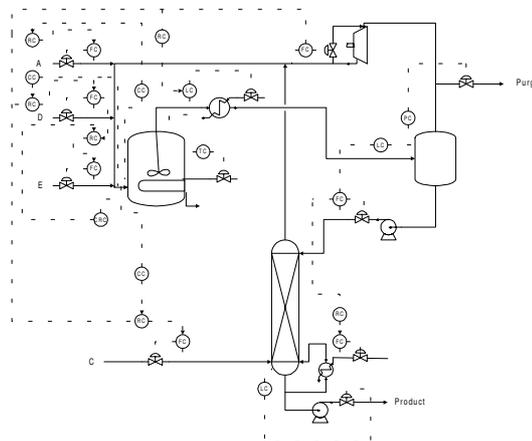
Fig. 9. Flowsheet of the control structure TE-CS1.
