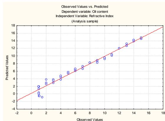
Fig. 9. Linear Regression – Refractive Index X Oil Content
