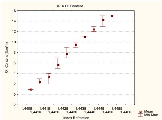
Fig. 5. Results of Index Refraction vs Oil Content
