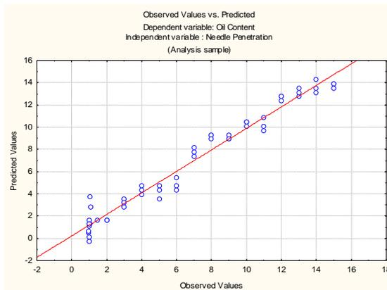
Fig. 12. Linear Regression – Needle Penetration vs Oil Content
