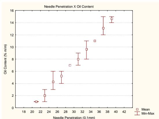
Fig. 8. Results of Needle Penetration vs Oil Content
