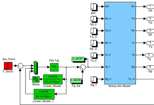
Fig. 1. Smith configuration for the rotary kiln control
