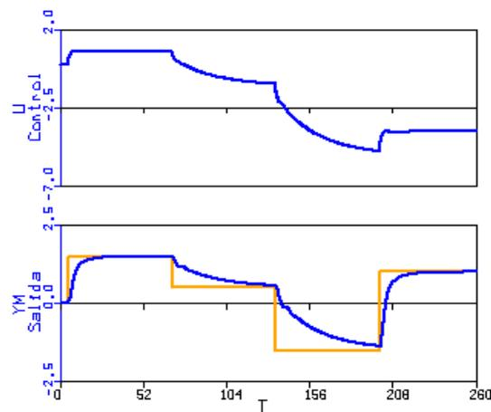
Fig. 12. Closed loop response of the asymmetric process to several step changes in the set point. Internal model  $G^+$  and  $\beta = 5$ . Upper graph: control signal. Lower graph: set point and process output.
