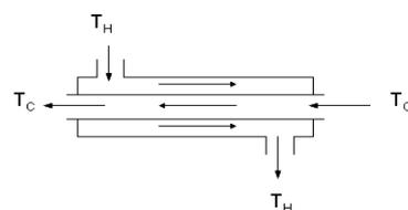
Fig. 2. Diagram of the countercurrent heat exchanger
