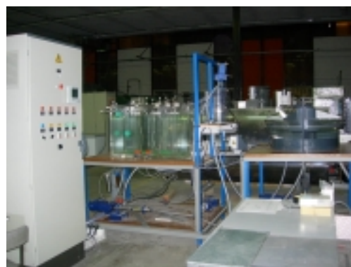
Fig. 1. The activated sludge pilot plant.
